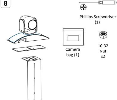
8. Attach camera to neck using supplied 1/4-20 bolt in camera hardware bag.
