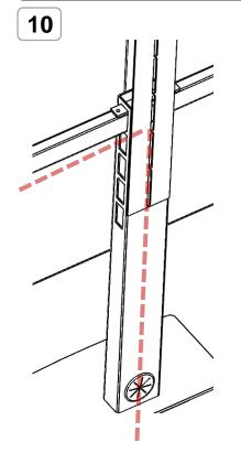
10. Run cables under tube and through main Pillar into furniture below or out rear grommet.
